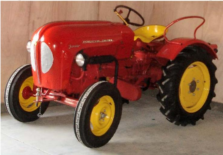
excellent condition. It has been well maintained and actually works well in the vineyard. It is a one cylinder diesel; it makes 12 horsepower, and has a top speed in 6<sup>th</sup> gear, of 12.5 MPH!
